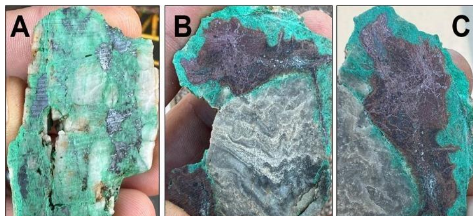
Rock Samples collected from Ellis Mine representing the brittle portion of a mineralized shear zone.
