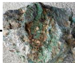
Grab sample of quartz sulfide vein with copper oxides and malachite
