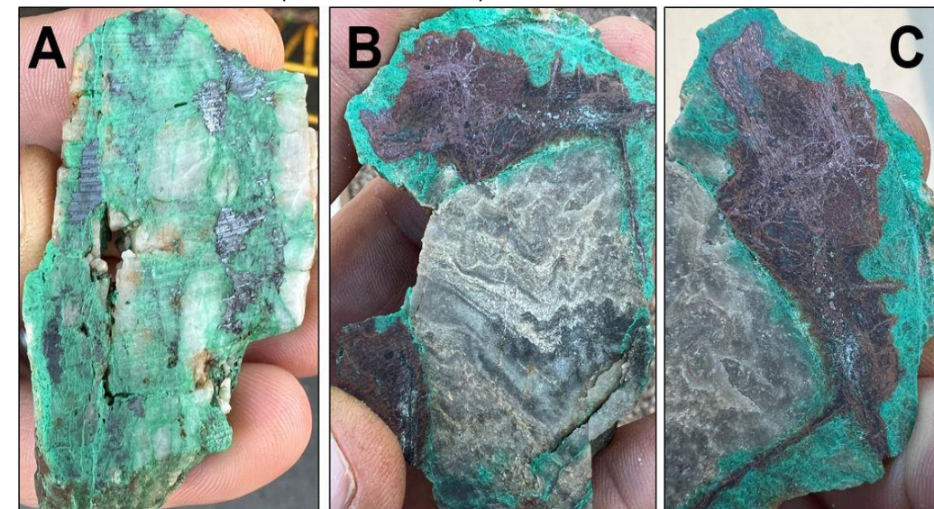
Rock Samples collected from Ellis Mine representing the brittle portion of a mineralized shear zone. A) Sheeted quartz veins with coarse euhedral bornite; B+C) Chrysocolla cemented breccia shows a shear-deformed clast rimmed by bornite and cuprite(?) with native copper.
