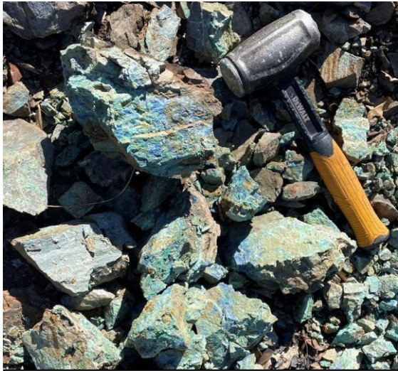
Dump sample of oxidized schist with disseminated malachite-azurite quartz-sulfide veinlets
