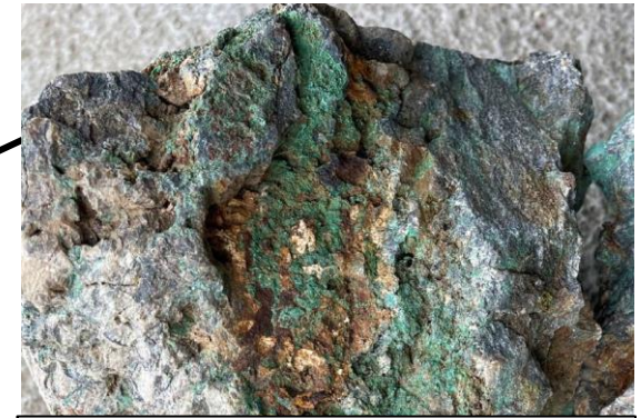
Grab sample of quartz sulfide vein with copper oxides and malachite
