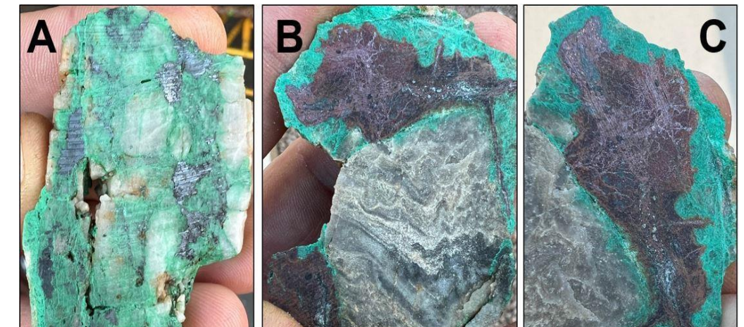
Rock Samples collected from Ellis Mine representing the brittle portion of a mineralized shear zone. A) Sheeted quartz veins with coarse euhedral bornite; B+C) Chrysocolla cemented breccia shows a shear-deformed clast rimmed by bornite and cuprite(?) with native copper.
