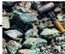
Dump sample of oxidized schist with disseminated malachite-azurite quartz-sulfide veinlets
